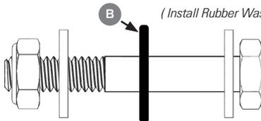
1/4" X 1-3/4" Hex Bolt - Rubber Washer - 1/4" Flat Washer (x2) - 1/4" Nyloc Jam Nut
