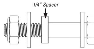
1/4" X 1-1/2" Hex Bolt - 1/4" Flat Washer (x2) - 1/4" Spacer - 1/4" Nyloc Jam Nut
