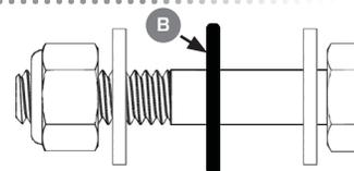
1/4" X 1-1/2" Hex Bolt - Rubber Washer - 1/4" Flat Washer (x2) - 1/4" Nyloc Nut
