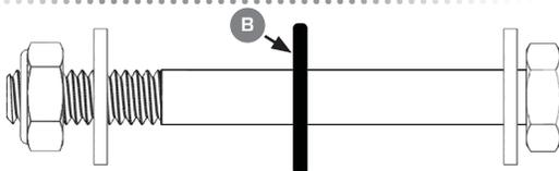
1/4" X 2-1/2" Hex Bolt - Rubber Washer - 1/4" Flat Washer (x2) - 1/4" Nyloc Jam Nut
