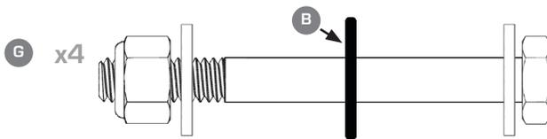
1/4" X 2-1/2" Hex Bolt - Rubber Washer - 1/4" Flat Washer (x2) - 1/4" Nylon Nut
