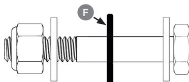
1/4" X 1-3/4" Hex Bolt - Rubber Washer - 1/4" Flat Washer (x2) - 1/4" Nyloc Nut
