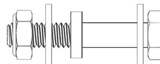
1/4" X 1-1/2" Hex Bolt - 1/4" Flat Washer (x2) - 1/4" Spacer - 1/4" Nyloc Jam Nut
