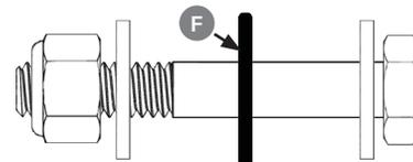
1/4" X 1-3/4" Hex Bolt - Rubber Washer - 1/4" Flat Washer (x2) - 1/4" Nyloc Nut
