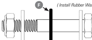
1/4" X 1-3/4" Hex Bolt - Rubber Washer - 1/4" Flat Washer (x2) - 1/4" Nyloc Jam Nut
