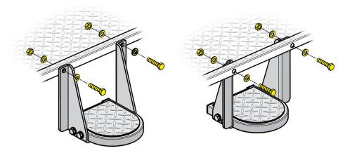
7. Hand tighten any loose hardware.
