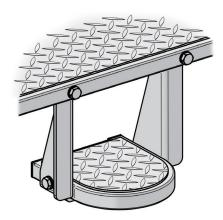
Fasten the mounting brackets to the step plate in the preferred orientation using (4) <u>M10 x 45mm Hex Head Bolts</u>, (8) <u>Flat Washers</u> and (4) <u>Nylock Nuts</u>. Tighten until snug but do not fully tighten.
