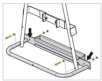
Fasten the lower bag support to the A-frame using (2) <u>M6 x 30 Button</u> <u>Head Cap Screws</u>, (4) <u>M6 Flat</u> <u>Washers</u> and (2) <u>M6 Nylock Nuts</u>. Hand tighten.
