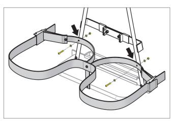
Fasten the vertical bracket on the lower bag support to the base frame using (1) <u>M6 x 30</u> <u>Button Head Cap</u> <u>Screw, (2) M6 Flat</u> <u>Washers</u> and (1) <u>M6 Nylock Nut</u>. Hand tighten.
