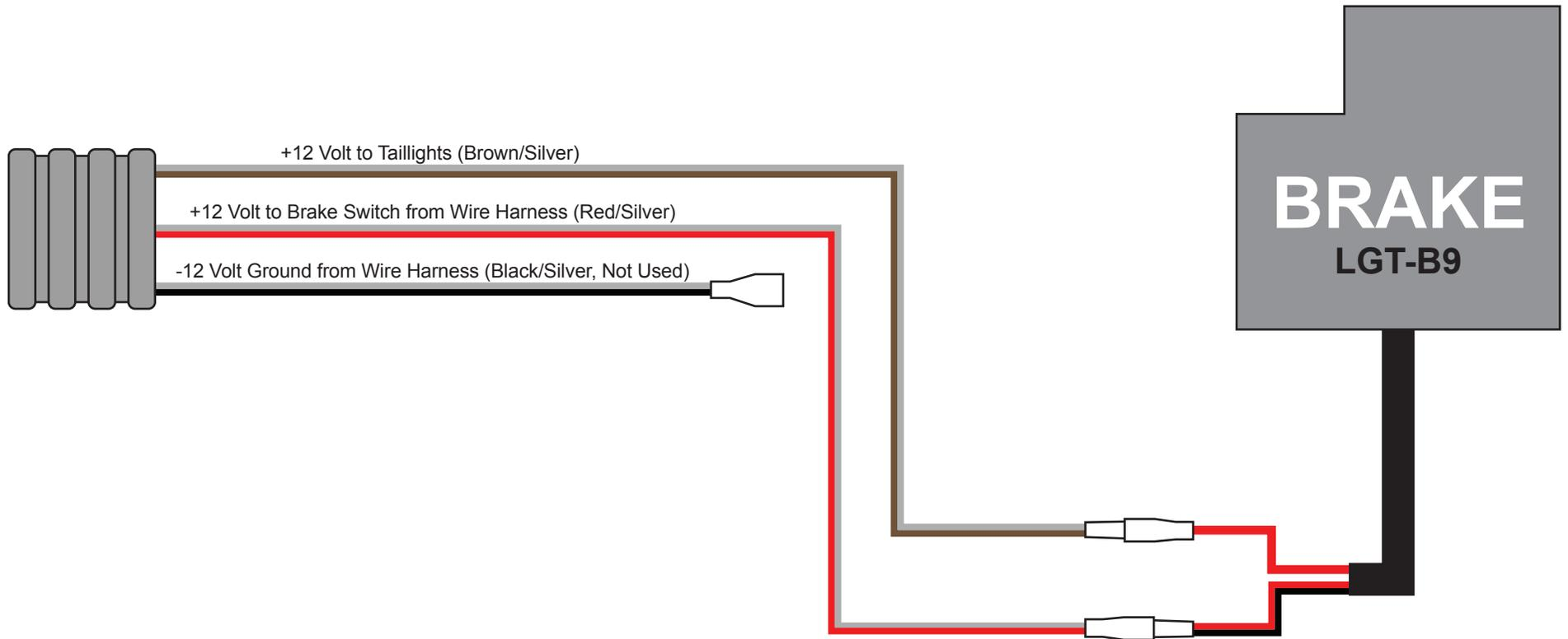
NOTE: The LGT-B9 connects directly to the bucket harness without the need for a subharness.
