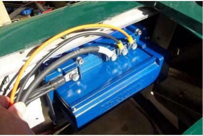
**10. The 16 pin control cable will be short.** Open the wire harness about 2-3 inches, install new zip ties or re-tape once the wire loom provides enough slack. In this example 2 inches of split loom were removed.
