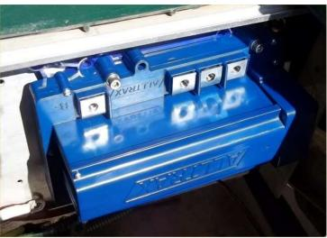
**8. B- WIRE is SHORT.** The Battery Minus wire that passes through the OBC computer will be 1/2- to 1" short, install the supplied 250 or 400amp fuse in the Battery Minus lead to add enough wire length.
