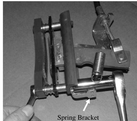
Fig R7 – Caliper re-assembly
