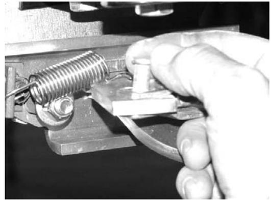
Fig. 11 - Attach brake cable to lever
