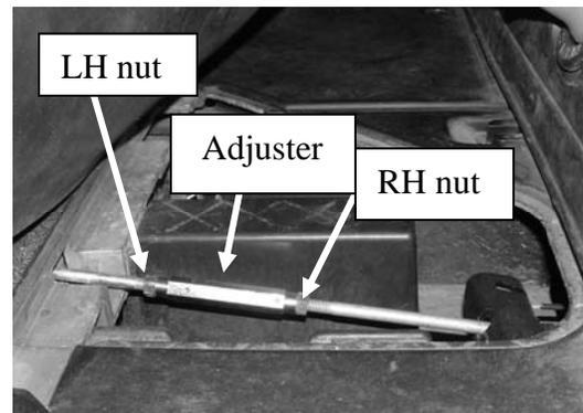
Fig R2 – Precedent cars – cable adjustment
