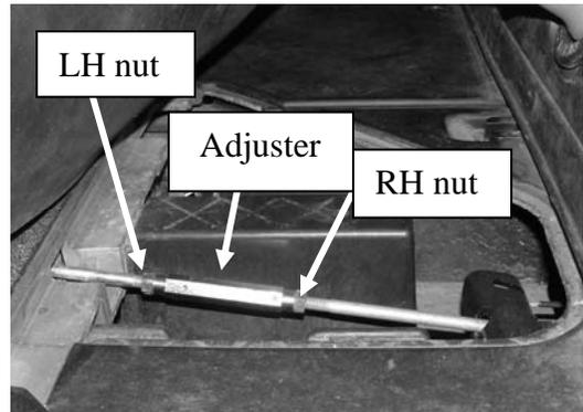
Fig M3 – Precedent cars – cable adjustment
