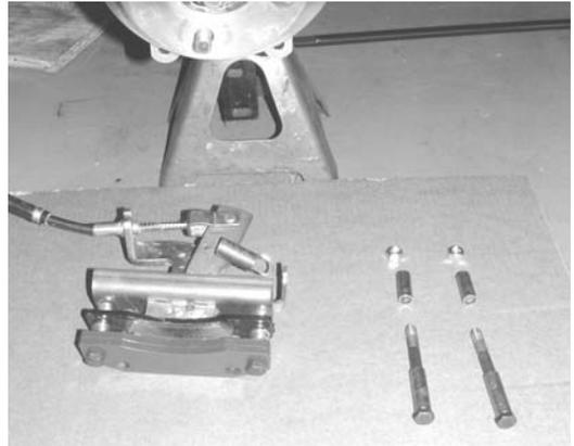
Fig R4 – Remove caliper.
