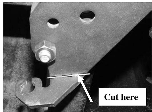
Fig 3 Original cable bracket
