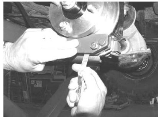
Fig. R8 - Check pad clearance
