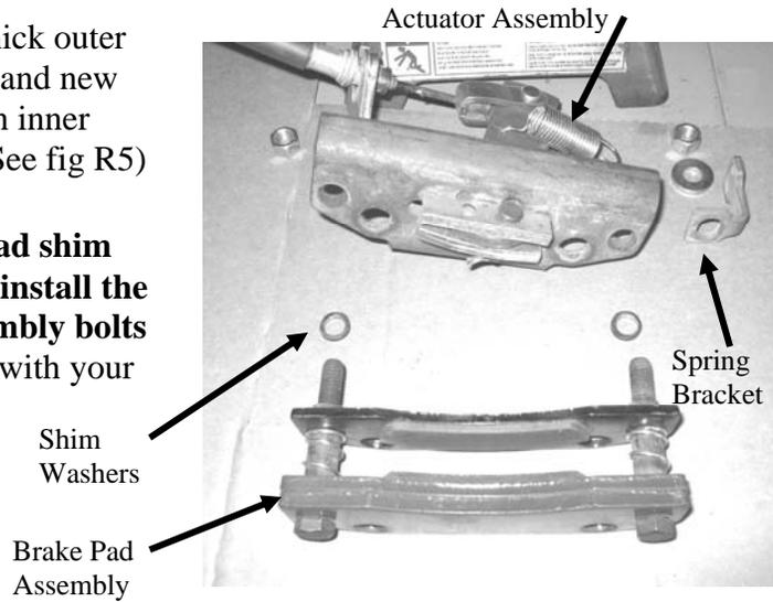
Fig R6 – New component assembly
