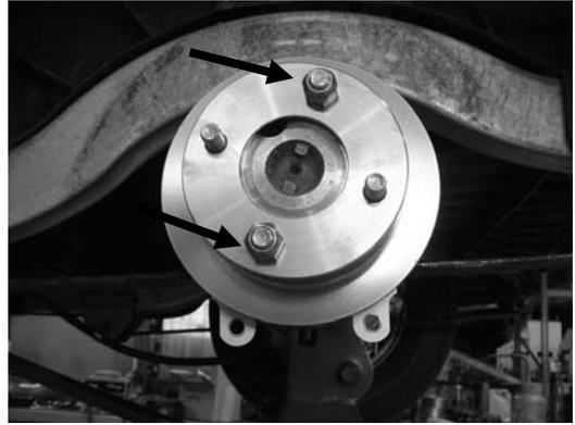
Fig R3 – Install 2 lug nuts.
