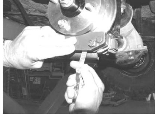
Fig. 14 Check pad clearance of both wheels at the same time.
