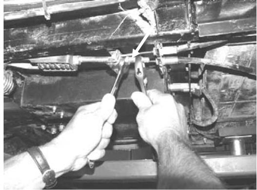
Fig. M2 – DS Cars – cable adjustment.
