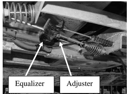
Fig. 12 – DS Cars – cable adjustment.
