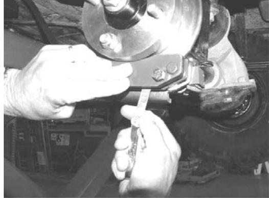
Fig. M4 Check pad clearance of both wheels at the same time.
