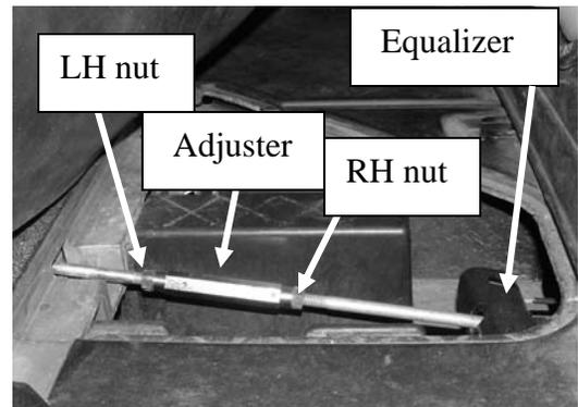
Fig 13 – Precedent cars – cable adjustment
