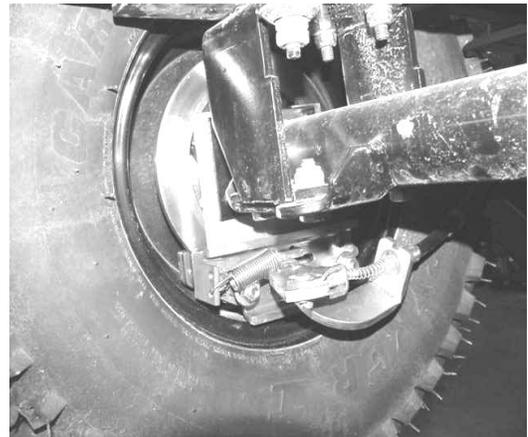
Fig 15 – Brake inside wheel
