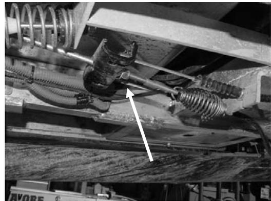
Fig. R1 – DS Cars – cable adjustment.
