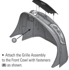
NOTE: Hand-tighten Hardware only. Over-torquing can pull threaded inserts out of plastic light bezels.
