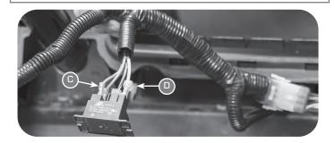
• Connect the Turn Signal 9-Pin Connector (C) to the Dash Harness 9-Pin Connector (D).
