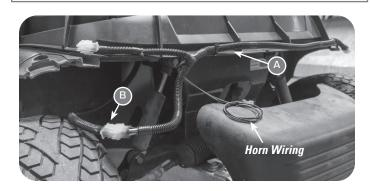
• The two remaining 6-Pin Connectors on the Headlight Harness connect to the Headlights. The Headlights will be connected and tested in Step 8.
