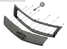
• Attach the Grille Insert to Grille Frame with fasteners (**C**) as shown.
