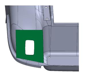
PLACE TEMPLATE ON CORNER OF BODY AS SHOWN. CUT HOLE IN BODY BEFORE PLACING ON CAR. FLIP TEMPLATE FOR USE ON OPPOSITE SIDE.
