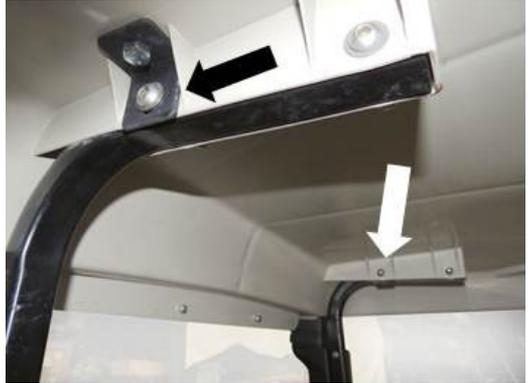
7. Identify (1) Rear Mounting Bracket. Position the Bracket so the larger hole touches the Top and place it over the newly drilled hole in the Top. The tab with the smaller hole should face the rear of the cart.
