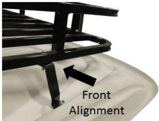
2. Once the Brackets are aligned, mark the hole locations on the underside of the square tubing of the Roof Rack for the Front Mounting Bracket holes.
