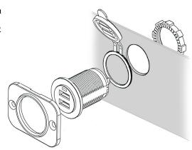
5. Use (2) spade connectors (not included) to connect your wires to the back of the outlet. Connect the positive (+) wire to the positive (+) terminal and the negative (-) wire to the negative (-) terminal. Terminals are marked positive (+) and negative (-).
