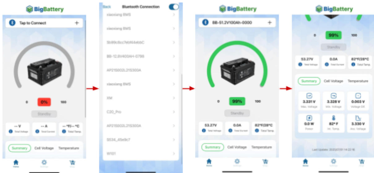
Figure 8: App and HUSKY2 Battery Connection
