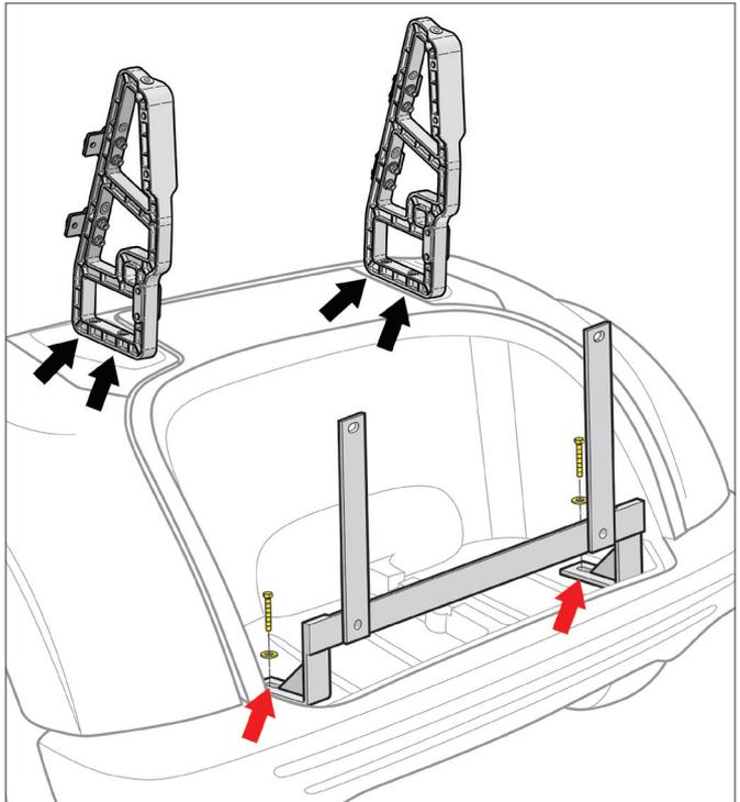
4. Install the sub-assembly brackets and the platform support bracket to the platform using using (2) M10 x 35 Hex Head Bolts, (4) Flat Washers and (2) Nylock Nuts (Bag #2). Hand tighten enough so the brackets are snug but still adjustable.
