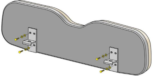
16. Install the rear seat back assembly to the rear seat back support frame using (2) M10 x 45 Hex Head Bolts, (4) Flat Washers and (2) Nylock Nuts (**Bag #5**).
