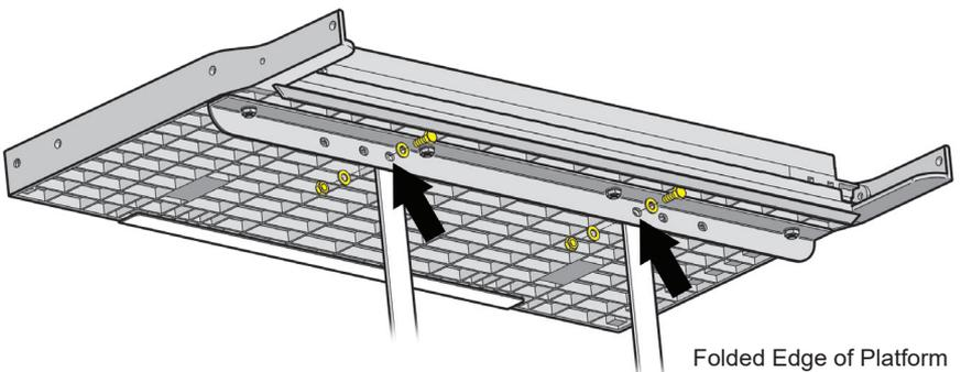
7. Loosely fasten the footplate to the vertical support bracket using (2) M10 x 35 Hex Head Bolts, (4) Flat Washers and (2) Nylock Nuts (**Bag #3**).
