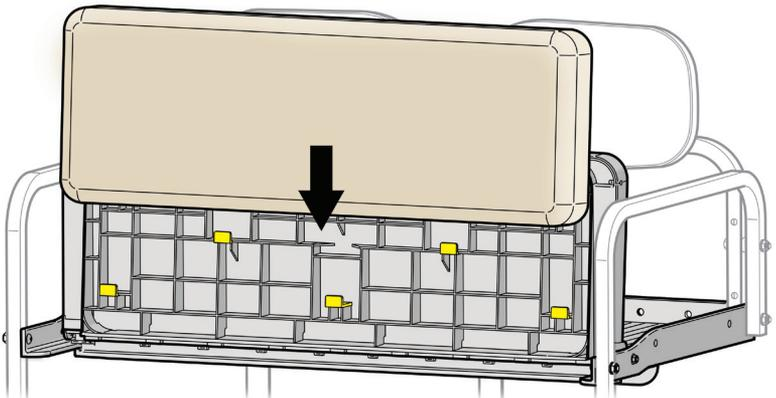
18. Fasten the handle to the seat platform using (2) M6 x 20 Phillips Head Countersunk Screws (Bag #5). Hand tighten to lock the seat bottom into place.
