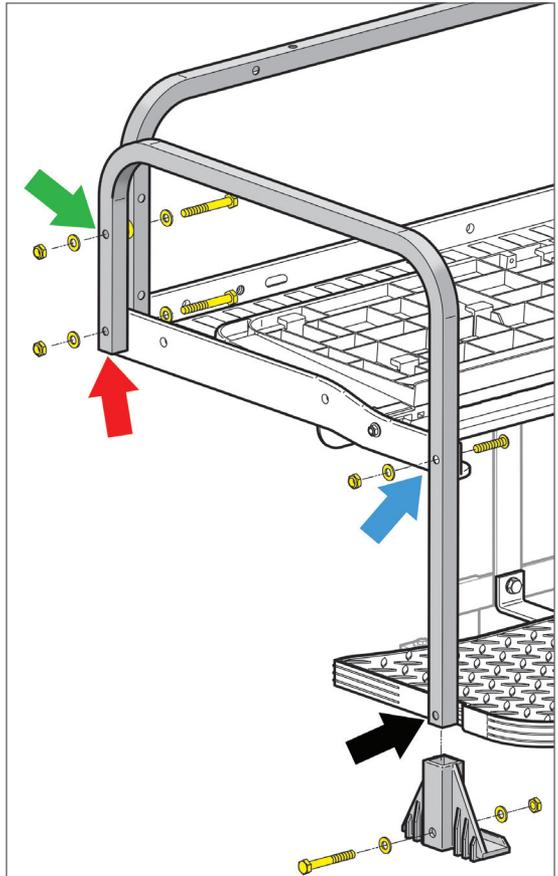
12. Loosely fasten the top of the handrails to the support frame (green arrow, page 6) using (2) M10 x 75 Hex Head Bolts, (4) Flat Washers, (2) Nylock Nuts and (2) Spacers (**Bag #4**).
