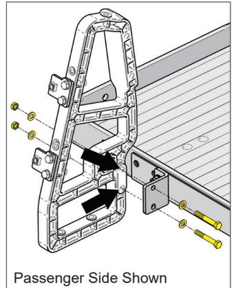
6. With the platform folded, loosely install the seat platform to the vertical support bracket using (2) M10 x 25 Hex Head Bolts, (4) Flat Washers and (2) Nylock Nuts (Bag #2).
