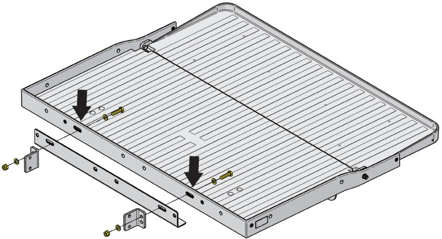
5. Loosely install the seat platform sub-assembly to the front seat back support brackets using (4) M8 x 55 Hex Head Bolts, (8) Flat Washers and (4) Nylock Nuts (Bag #2).
