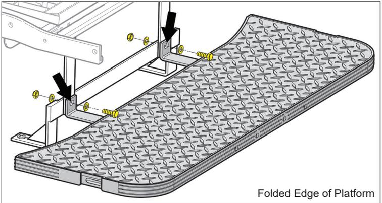
8. Loosely fasten the longer leg of (1) handrail to the rearmost portion of the seat platform (blue arrow) using (1) M10 x 45 Phillips Head Truss Bolt, (1) Flat Washer & (1) Nylock Nut (**Bag #4**).
