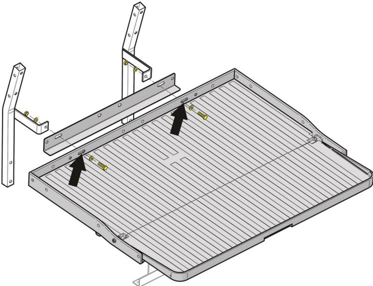
7. With the platform folded, loosely install the seat platform to the vertical support bracket using (2) 10mm x 25 Hex Head Bolts, (4) Flat Washers and (2) Nylock Nuts (**Bag #2**).
