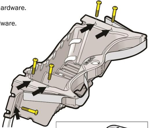
9. Remove both seat back support brackets and rubber boots. The brackets are attached to the frame, under the body.
