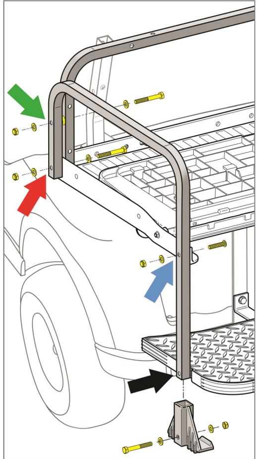
16. Install the rear seat back brackets to the rear seat back using (4) 6mm x 25 Hex Head Bolts, (4) 6mm Lock Washers and (4) 6mm Flat Washers (**Bag #5**). Hand tighten.
