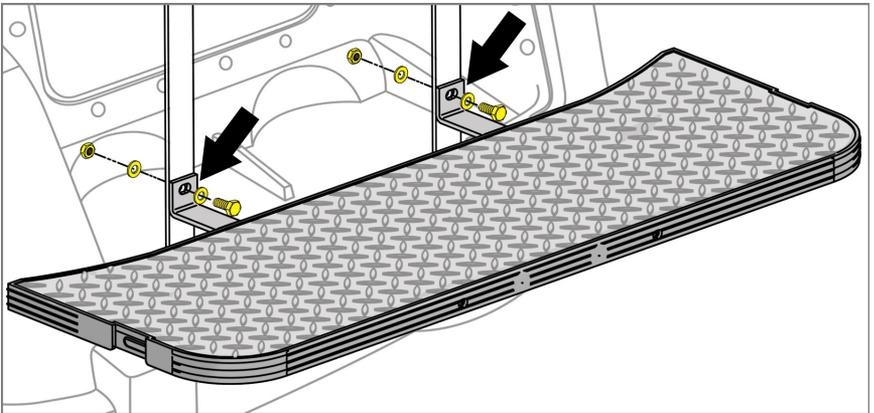
9. Loosely fasten the longer leg of a handrail to the rearmost portion of the seat platform (blue arrow, page 7) using (1) 10mm x 45 Phillips Head Truss Bolt, (1) Flat Washer and (1) Nylock Nut (**Bag 4**).
