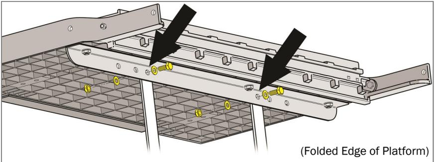
8. Loosely fasten the footplate to the vertical support bracket using (2) 10mm x 35 Hex Head Bolts, (4) Flat Washers and (2) Nylock Nuts (**Bag #3**).
