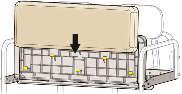
19. Fasten the handle to the seat platform using (2) 6mm x 20 Phillips Head Countersunk Screws (**Bag #5**). Hand tighten to lock the seat bottom into place.
