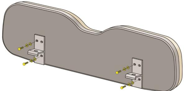
17. Install the rear seat back assembly to the rear seat back support frame using (2) 10mm x 45 Hex Head Bolts, (4) 10mm Flat Washers and (2) 10mm Nylock Nuts (**Bag #5**).
