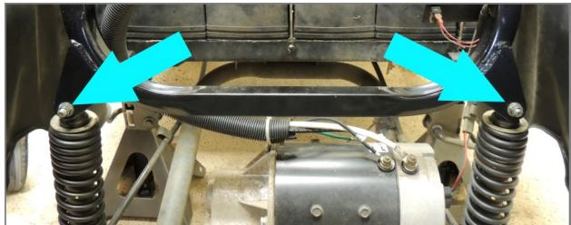
9. Reroute and reconnect the wire disconnected in step 4. Use a wire tie to secure it if needed.
