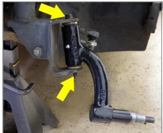
3. Attach the steering knuckles to the spindles using the Original Hardware.
