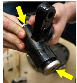
2. Install the new spindles to the spindle mounting area on the shocks using the Original Hardware. Driver side is shown.
