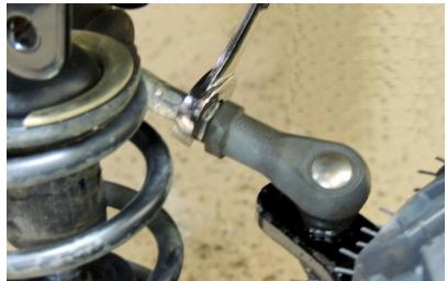
4. Once toe adjustments are finalized and set, tighten all hardware and jam nuts.
