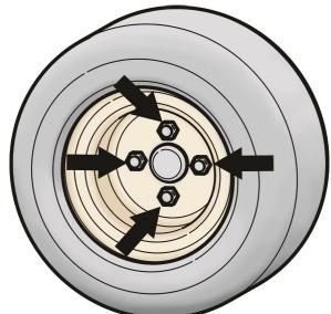
8. Remove the dust caps from the hubs. Remove the hubs from the spindles. Retain dust caps, hubs and hardware.
