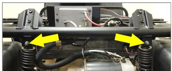
4. Disconnect the pin connector attached to the motor to eliminate damage when lowering the rear suspension (electric carts only).
