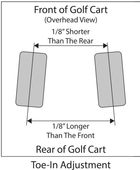
3. Adjust the toe by loosening the jam nut then lengthen or shorten the tie rod by turning the hex shaped rod adjustment. Shortening the tie rods increases the toe-in, lengthening decreases it.
