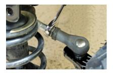
Once toe adjustments are finalized and set, tighten all hardware and jam nuts.
