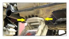
2. Disconnect the rear connecting rod by removing the (2) bolts, nuts and washers. Retain rod and hardware.
