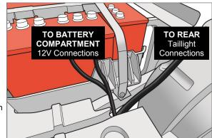
5. Feed the rear portion of the harness through the cart so the taillight connections reach the holes in the rear body. The shorter cable will rest on top of the driver side fender. Route the longer cable behind the battery compartment and over the passenger side rear fender.
