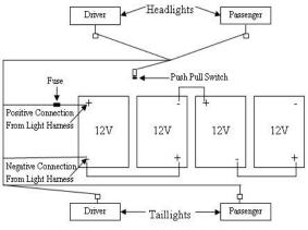
Yamaha 48 Volt System with 12 Volt Batteries
