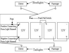
Yamaha 48 Volt System with 12 Volt Batteries
