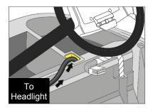
3. If powering the lights with a push-pull switch, locate the indentation to the right of the key switch on the dash panel and drill a 7/16" hole. File any rough edges.
