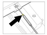
Slide the small brake switch bracket upward, between the nut and rod. Tighten the nut. Disengage the brake pedal.
