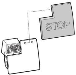
2. Reinstall the new brake pad by fitting it over the plate where the OE brake pad was removed.
