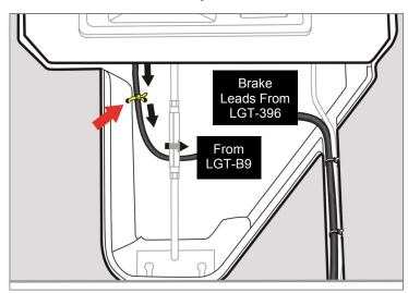
Connect the brake pad to the brake leads from the bucket harness (LGT-396 or OE harness). Use cable ties to secure loose wires away from any moving parts.
