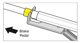
3. Mount the brake switch towards the rear of the pedal compartment with the included <u>Self-Tapping Screws</u>. Position the switch so the spring is tight but not pulling the plunger (red arrow, Page 19). The plunger should move to activate the switch when the brake pedal is engaged. Unscrew the rear portion of the switch if needed for clearance.
