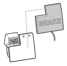
3. With the brake pedal in PARK, run the wire from the pad down the left side of the pedal and into the pedal compartment. Keep the wire close to the driver side so it does not get pinched.
