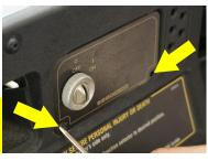
1. If powering the lights with the <u>push-pull</u> switch, disconnect the key switch. Using a vice or clamp to secure the plate, safely drill a 1/2" hole on the key switch plate. File any rough edges.
