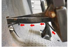
Connect the brake pad to the deluxe wire harness. Use a cable tie to secure the wires to the existing wire harness in the channel. Make sure the wires are clear of any moving parts.
