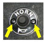
10. Connect the (2) ring terminals from the horn harness to the back of the horn button. You can connect the leads to either terminal.
