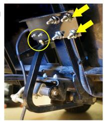
Position the bracket so the switch is centered above the pedal assembly. Lower it until the switch is activated (it will click).
