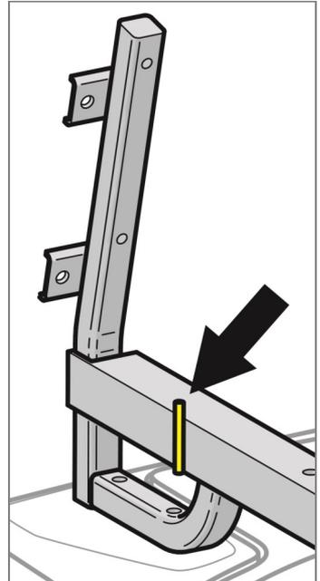
7. Fasten the utility box to the support frames using (4) 10mm-1.5 x 35mm Phillips Head Truss Bolts, (4) 10mm Flat Washers and (4) 10mm-1.5 Nylock Nuts.
