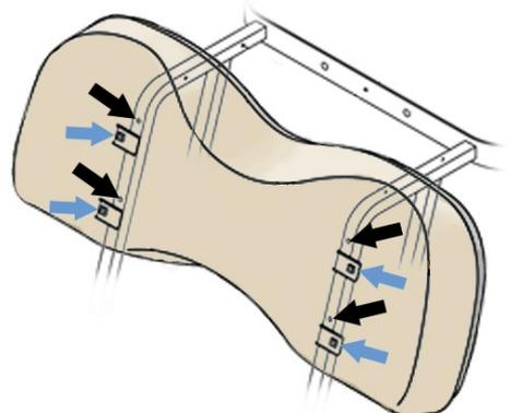
9. Remove the seat back support and the bag attachment assembly. Retain hardware.
