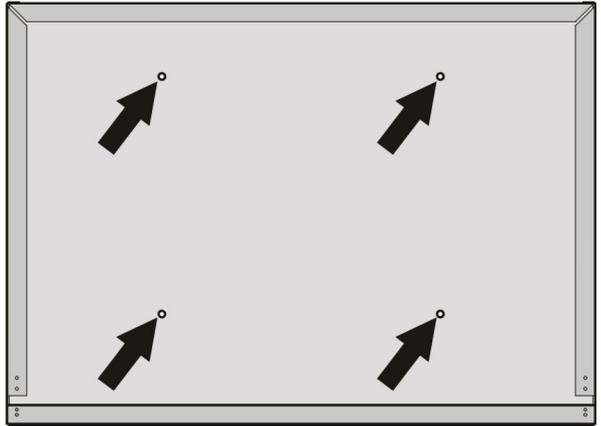
8. Fasten the latch catches to the tailgate using (2) 10-32 x 1" Pan Head Phillips Machine Screws, (2) Flat Washers and (2) Nylock Nuts (black arrow).
