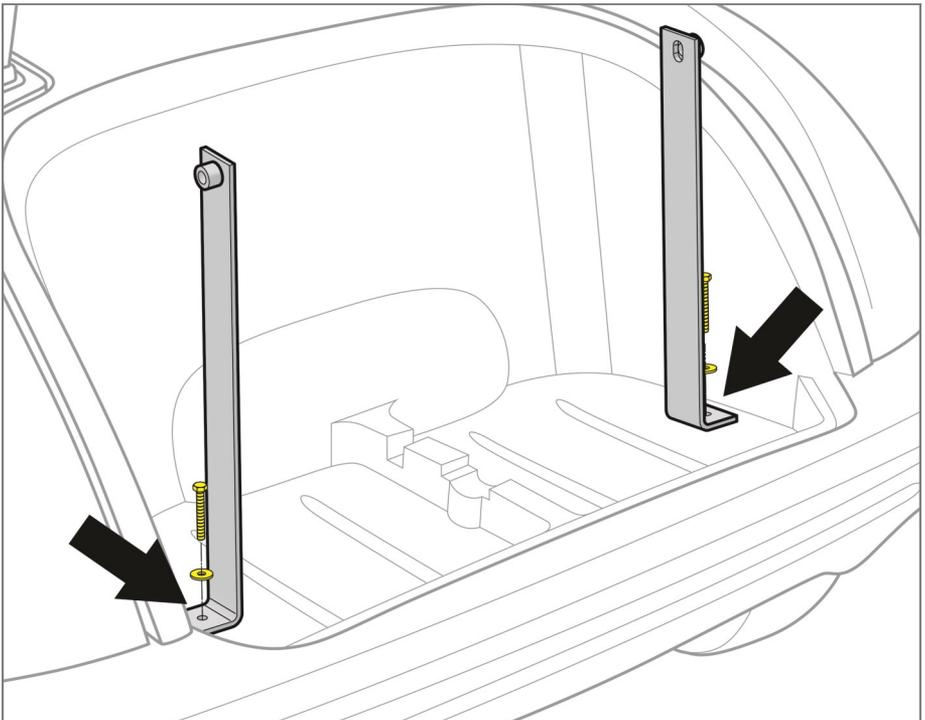
3. Install the utility box support frames to the rear body where the seat back support was removed. Mount using the Original Hardware. Place an end cap on the upper open ends of the support frames.
