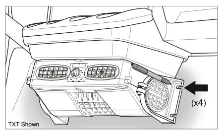
Using a marking device, mark a hole location in the center of the (4) marked holes. This will be used to route the wires into the battery compartment.
