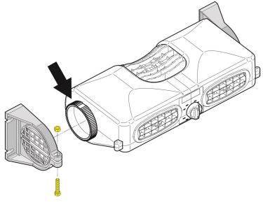
2. Place the fan in the desired mounting location. This location should be as far up on the floor board as possible. Once the fan is in the correct location, mark the center of the (4) mounting holes with a marking device.
