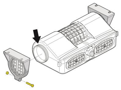
Locate an area on the top to install the fan. Use a tape measure to make sure the fan is centered and the brackets are square. Once the fan is in the desired location, mark the center of the (4) mounting holes with a marking device.
