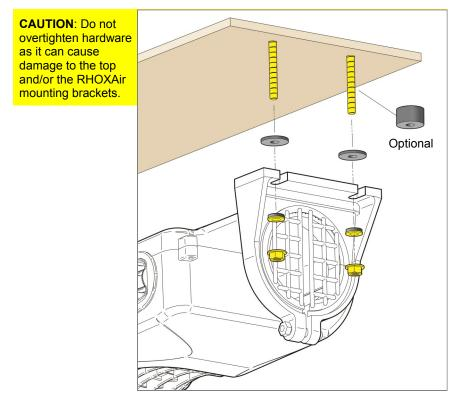
6. Use an oscillating or reciprocating saw to trim off any excess bolt length from the (4) mounting bolts. Leave at least a 1/4" of exposed threads on the bolt.
