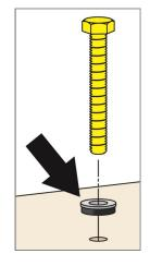
Place the (4) <u>Rubber Washers</u> between the top and the fan as shown. Install the RHOXAir fan to the top using (4) <u>6mm Serrated Flanged Locknuts</u> and (4) <u>6mm Metal Bonded Sealing Washers</u>. Use the <u>6mm x 13mm Thick</u> <u>Rubber Spacers</u> to provide more angle if needed. Hand tighten hardware.
