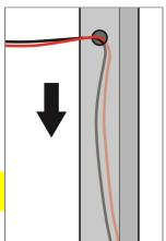
Make sure the wires can reach the power source. Trim off any excess length if needed. Attach the <u>Male Spade Connector</u> to the red wire (+12V or 48V) coming out of the fan. Attach the <u>Ring Terminal</u> to the black wire (-12 or 48V).
