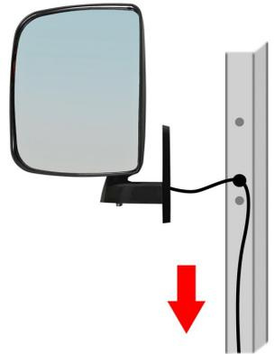
9. Use the included mounting hardware to mount the mirror to the strut. Do not over tighten the mounting screws.
