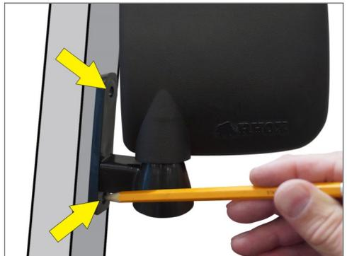
3. Use an 1/8" drill bit to drill the top and bottom marked hole locations on the driver side strut. Do NOT drill completely through the strut. Only drill through the first wall.
