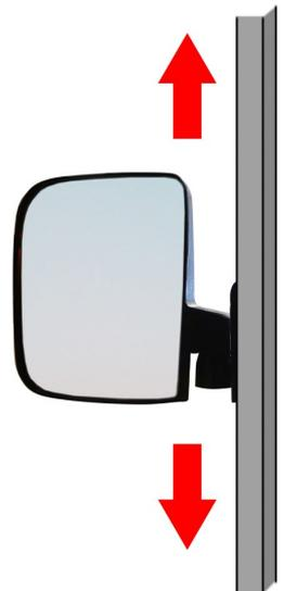
2. With the mirror in the correct position, use a marking device to mark the location of the mounting holes on the driver side front strut. Set the mirror in a safe location.
