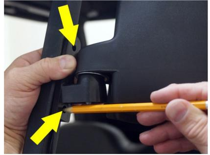
3. Use an 1/8" drill bit to drill the top and bottom marked hole locations on the driver side strut. Do NOT drill completely through the strut. Only drill through the first wall. File or sand any rough edges.
