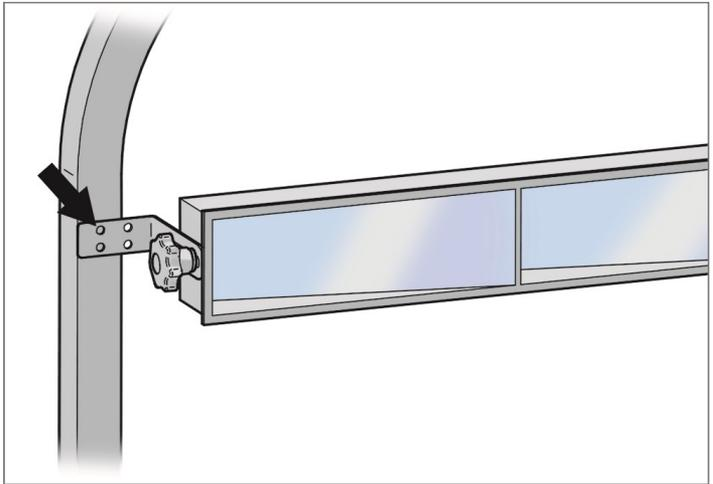
4. Using a 1/16" drill bit, drill a pilot hole at the marked location.
