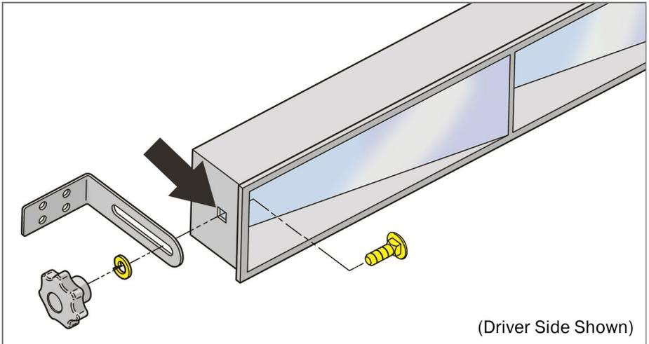
2. Position the mirror evenly on the front strut(s) in a convenient location for the driver. The brackets are universal and can be mounted to the vertical or horizontal portion of the strut(s).
